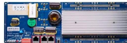
RS485 Communication between battery and inverters Stand rate:9600bps RS485 Interface Communication between parallel packs or BMS and PC Stand rate:9600bps
