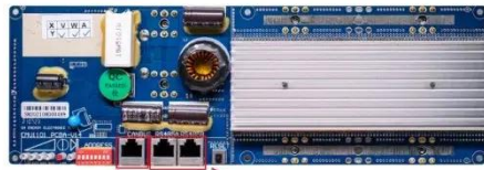
RS485 Interface Communication between parallel packs of BMS and PC Band rate:9600bps
