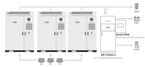
Application scenarios of energy storage battery products
