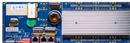
RS485 Communication between battery and inverters Band rate:9600ps RS485 Interface Communication between parallel packs of BMS and PC Band rate:9600ps
