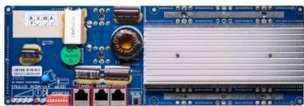
RS485 Communication between battery and inverters Board size: 90x90mm RS485 Interface Communication between parallel packs of BMS and PC Board size: 90x90mm
