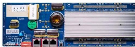
RS485 Communication between battery and inverters Band rate:9600ps RS485 Interface Communication between parallel packs of BMS and PC Band rate:9600ps
